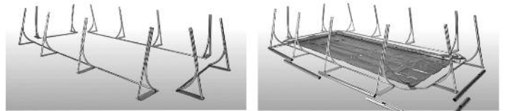
1 Assembly of the legs and the lower parts of the metal frame.
